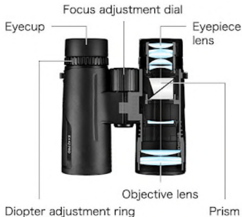
Anatomy of a Binocular (Pic courtesy: Olympus Asia)
